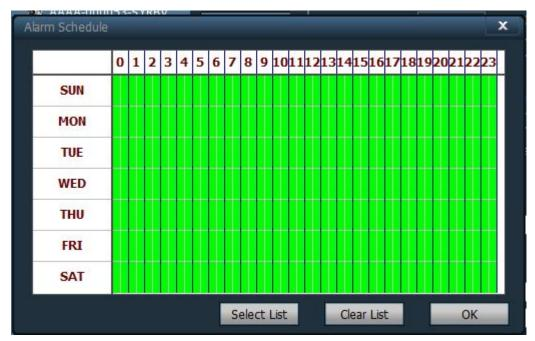
SUN – SAT means one week, based on the count of day; 0 – 23 means one day, based on the unit of half an hour.
