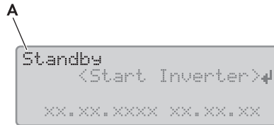
Figure 6: Display of operating states (example "Standby")
