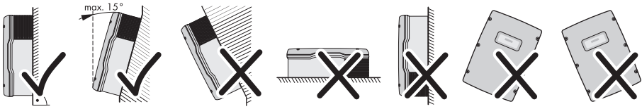
Figure 11: Permitted and prohibited mounting positions
